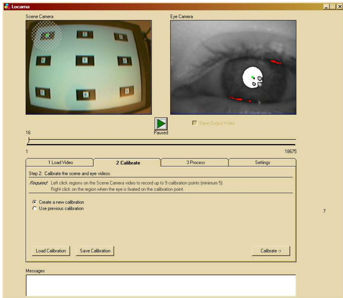
Fig. 4 Locarna Eye Gaze Calibration. The eye is focused on the first point, which is selected.
